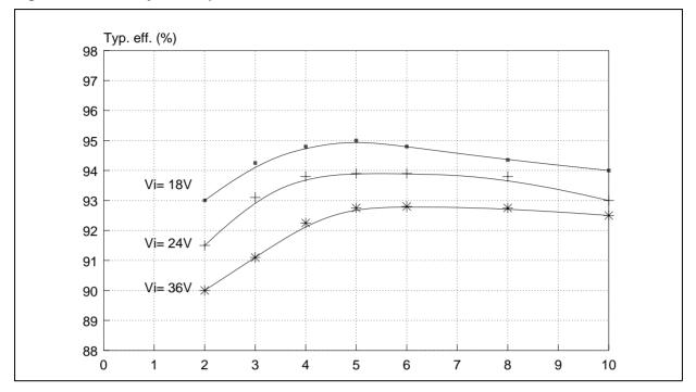
Figure 5. - Efficiency vs. Output Current.
